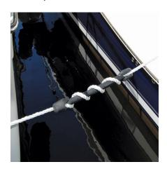
Snubbers absorb shock and will help extend the life of your dock lines while minimizing stress to structural areas around cleats caused by the jolting action of wind, waves, and wakes. Even with the attenuator project near completion the marina will still experience wave action that will put stress on the dock lines, boats, and docks. Every boat should have
